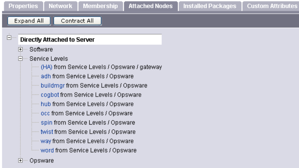
Figure 8-21: Nodes Tab That Shows the Service Level to Which a Server is Assigned
