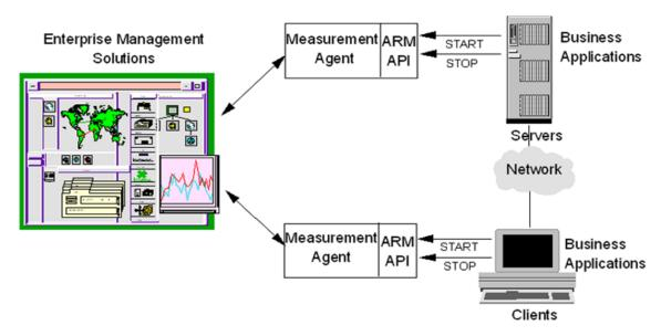
Figure 1 shows how enterprise management applications, measurement agents that implement the ARM API, and business applications that call the ARM API work together to provide a robust way to monitor application response.
