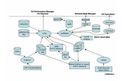
Figure 2 Component interaction with DCE or NCS mode enabled
