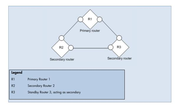
**Scenario**: A Router Redundancy Group has multiple routers reporting as the secondary router. A properly functioning HSRP or VRRP Router Redundancy Group should have only one operational secondary router.
