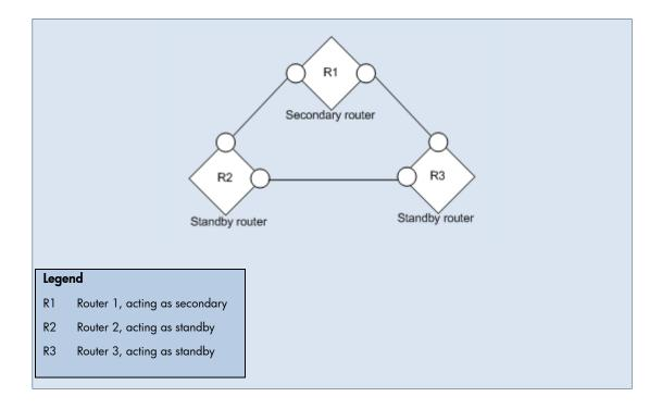
**Scenario**: A Router Redundancy Group does not have a primary member. A properly functioning HSRP or VRRP Router Redundancy Group should have one operational primary router and one operational secondary router.
