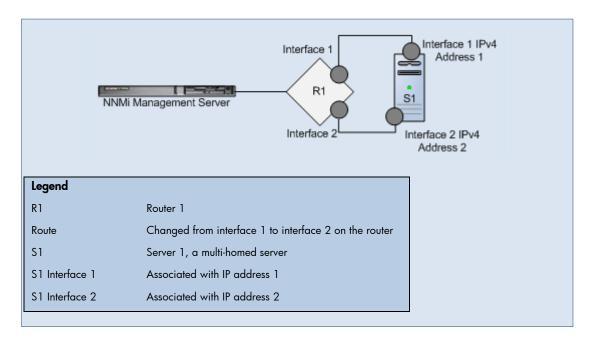
**Scenario**: IP address 1 on Server 1 (S1) is not responding. For example, the route on Router 1 (R1) has changed from Interface 1 to Interface 2, so that packets destined for the interface 1 on Server 1 are now routed out of Interface 2 on Router 1. The associated interface is operational, and the node can be reached because you can ping some IP addresses. The SNMP agent is up.
