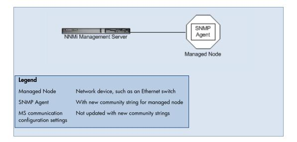
**Scenario**: The SNMP agent is not responding. For example, the community string for this SNMP agent has been changed, or NNMi's communication configuration settings have not yet been updated, but the node is operational (IP addresses can be pinged).
