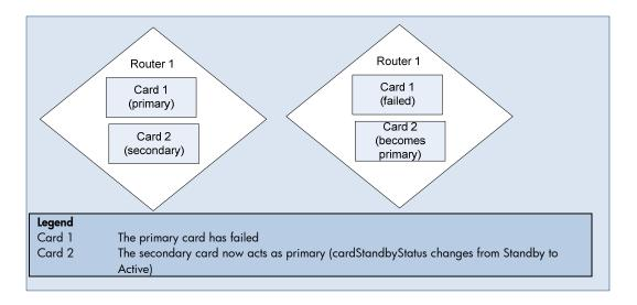
**Scenario**: A Card Redundancy Group has a failure on the primary card. The <code>cardStandbyStatus</code> on the secondary card changes from the value of Standby to Active. This Active card takes over as the primary member. In this case, the Card Redundancy Group is functioning as intended.
