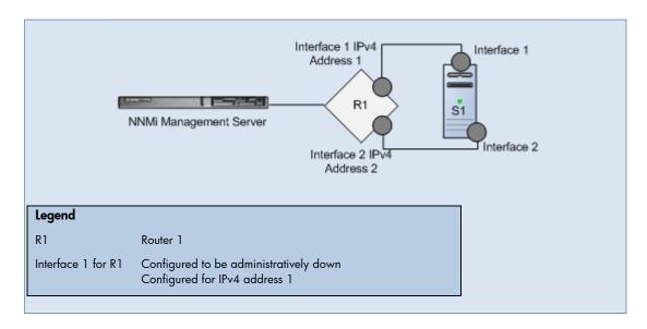
Scenario: Interface 1 on Router 1 is administratively down (ifAdminStatus = down), but the node (Router 1) can be reached. For example, Interface 2 responds to ping and the SNMP agent is up. Disabling Interface 1 brings that interface operationally down. The IP address associated with this interface, IP Address 1, stops responding to ICMP.
