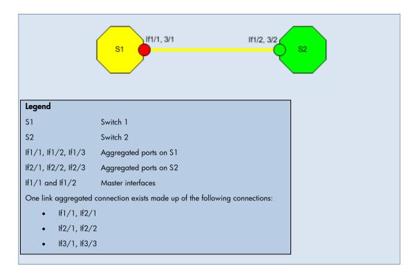
Scenario: All ports within the port aggregator are operationally down.
