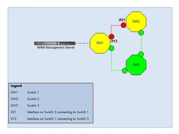
**Scenario**: The connection between the interface on Switch 3 connecting to Switch 1 (if13) and the interface on Switch 1 connecting to Switch 3 (if31) is down. Traffic flows from the Management Server through Switch 1 (SW1) and Switch 2 (SW2). Both if13 and if31 are marked down.
