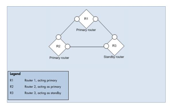
**Scenario**: A Router Redundancy Group has multiple routers reporting as the primary router. A properly functioning HSRP or VRRP Router Redundancy Group should have only one operational primary router.
