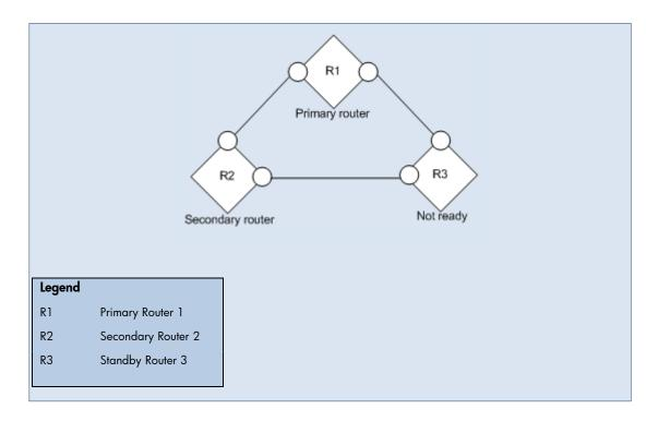
**Scenario**: The Router Redundancy Group has had some change. The group is functioning, and there are one primary router and one secondary router, but there is some non-normal condition that could be an issue. For example, there might be several routers not in a Standby state.
