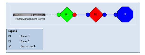
**Scenario**: There is no redundancy to Router 2 (R2). Either Router 2 is down or the connection between Router 1 (R1) and Router 2 is down.
