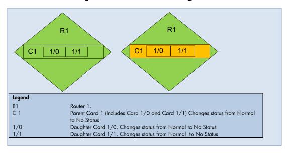
**Scenario**: Router 1 is managed and is polled. All cards on Router 1 are up. The Parent Card, Card 1, management mode is set to Unmanaged or Out-Of-Service.
