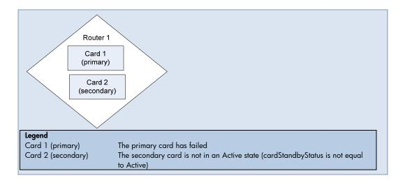
**Scenario**: A Card Redundancy Group does not have a primary member. The <code>cardStandbyStatus</code> of the primary card (Card 1) is not Active. Router 1 sends a <code>CiscoRFProgressionNotif</code> or a <code>CiscoRFSwactNotif</code> trap on the Card Redundancy Group state changes.
