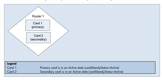
**Scenario**: A Card Redundancy Group has both members reporting as the primary card. The cardStandbyStatus of both cards is Active. A properly functioning Card Redundancy Group should have only one operational primary card.
