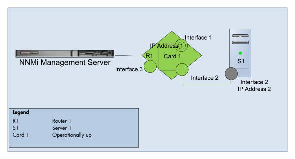
**Scenario**: This scenario continues the previous "Card is Operationally Down" scenario. Card 1 is operationally up (cardOperStatus = up). The node (Router 1) can be reached and all of its IP addresses respond to ping. The card is up and all the interfaces and connection on Card 1 are back to normal. The SNMP agent is up.
