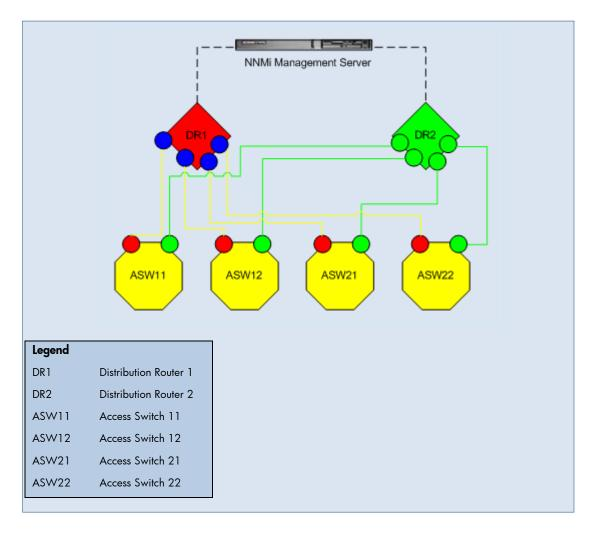
**Scenario**: Access switches ASW11, ASW12, ASW21, and ASW22 are redundantly connected to the distribution routers, as shown. The distribution routers DR1 and DR2 are directly connected to one another. The distribution router DR1 goes down.
