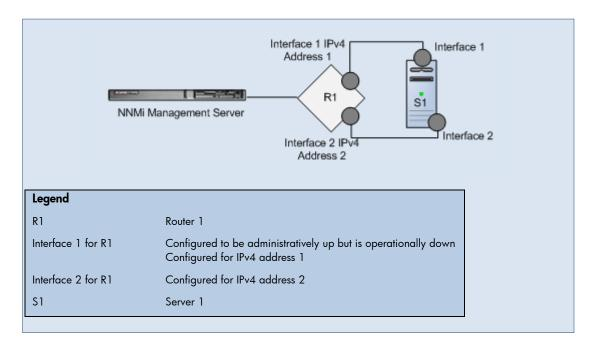
Scenario: Interface 1 is operationally down (ifOperStatus = down) and administratively up (ifAdminStatus = up). Router 1 sends a linkDown trap. Router 1 can be reached because some IP addresses, such as IP Address 2, respond to ping. The SNMP agent is up. IP Address 1 is associated with Interface 1. IP Address 1 has stopped responding to ICMP.
