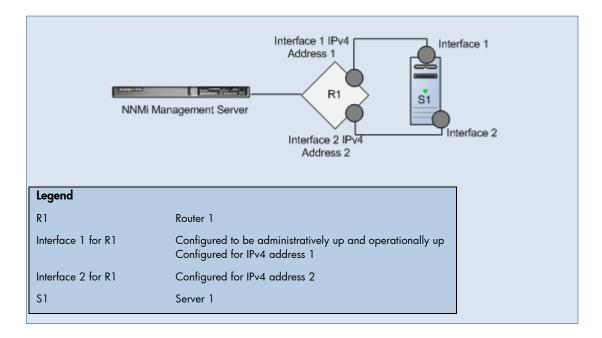
**Scenario**: This scenario continues the previous "Interface is Operationally Down" scenario. Interface 1 on Router 1 is now operationally up (ifOperStatus = up). The node can be reached. All of its IP addresses respond to ping. The SNMP agent is up.
