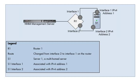
**Scenario**: This scenario continues the previous "IP Address Not Responding to ICMP" scenario. The IP address is now responding, the associated interface is operational, and the node can be reached. (For example, you can ping some IP addresses and the SNMP agent is up, or both.)
