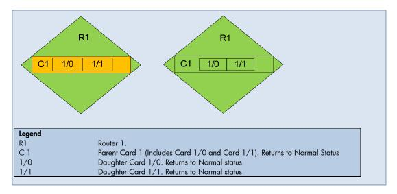
**Scenario**: This scenario continues the previous "Parent Card Management Mode is Unmanaged or Out-of-Service" scenario. The Parent Card management mode is now set to Inherited. This means the Parent Card's management mode is inherited from its container node (Router1), which is Managed.
