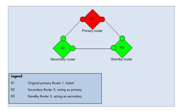
**Scenario**: A Router Redundancy Group has had a failure on the primary router and the secondary router has taken over as primary. Usually the standby becomes the secondary, which is not a problem. The group is functioning as intended. The incident generated for this scenario is for informational purposes to report that the group has had a failover.
