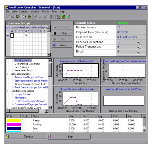
The following procedure outlines how to use the LoadRunner Controller to create, run, and analyze a scenario. For more information, refer to the *LoadRunner Controller User's Guide*.
