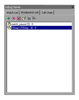
**Tip:** The Debug Viewer window can be displayed as a docked window within the WinRunner window, or it can be a floating window that you can drag to any location on your screen. By default the Debug Viewer opens as a docked window on the right side of the WinRunner screen. To move the window to another location, drag the Debug Viewer titlebar.
