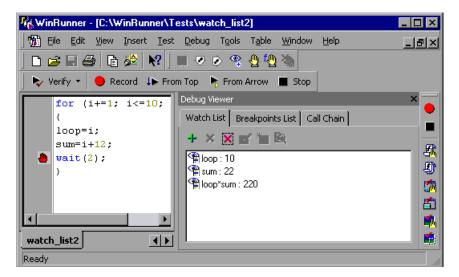
After WinRunner executes the first loop, the test pauses. The Watch List displays the variables and updates their values: When WinRunner completes the test run, the Watch List shows the following results:
