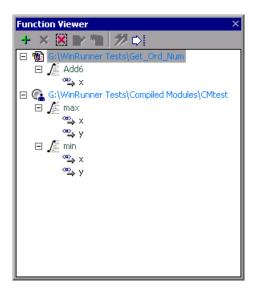
The Function Viewer is comprised of a toolbar and a pane that displays the function tree.
