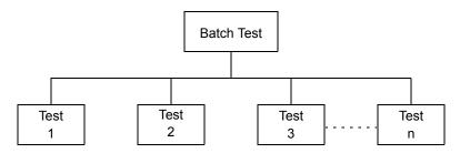
A batch test looks like a regular test that includes call statements. A test becomes a "batch test" when you select the **Run in batch mode** option in the **Run** category of the General Options dialog box before you execute the test.
