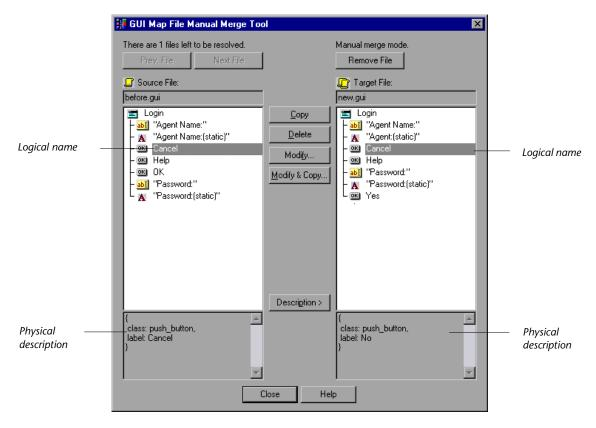
Note that in the above example, the highlighted objects in both panes have identical logical names but different descriptions. Therefore, they cannot both exist "as is" in the merged file.
