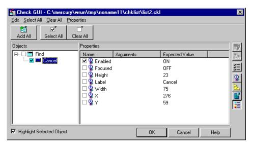
The following Check GUI dialog box displays a custom check as well as the standard checks for push\_button class objects:
