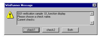
Dialog box with custom user interface developed using WinRunner's pause\_test function
