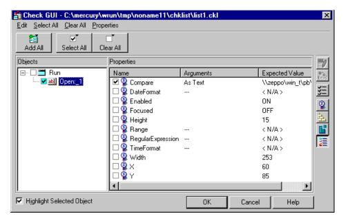
The following Check GUI dialog box displays a custom property check as well as the standard property checks for edit class objects:
