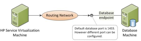
The default port of the database endpoint is **1433**. However, the database administrator can reconfigure the database to use a different port.
