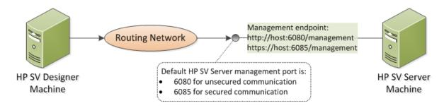
The Service Virtualization Designer also provides a management port, used mainly for connecting to integration testing tools.
