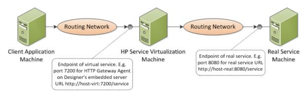
In this figure, the client application is reconfigured to communicate with the virtual service instead of the real service. The virtual service can be deployed on one of the following:
