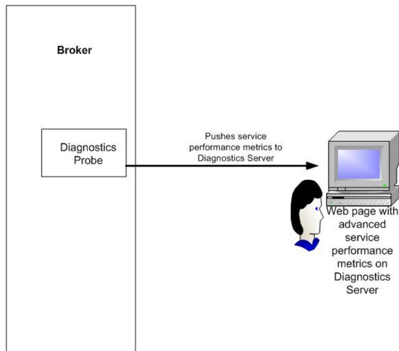
In the diagram, the SOA PE Broker is configured to integrate with Diagnostics Server. Therefore, the Diagnostics probe sends the service performance metrics from the Broker to the Diagnostics Server. This integration enables you to view the service performance metrics. See the HP Diagnostics documentation for more information about HP Diagnostics.
