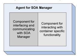
While designing and developing an agent, you must separate (abstract) the WS interfaces layer from the management functionality layer. This abstraction allows changes to one of these layers without affecting the other layer. This approach helps you to port the agent even when the WS interface to the SOA Manager is updated to evolving standards in future.
