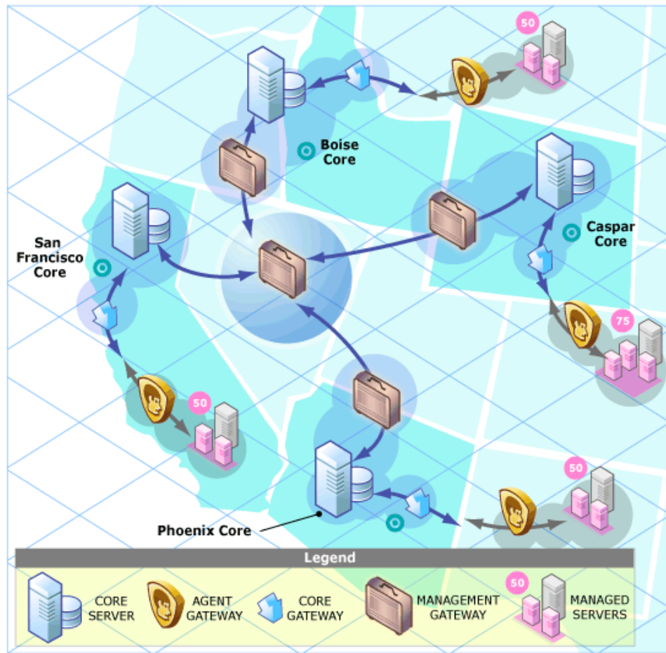
Figure 5 Multimaster Mesh with Four Cores
