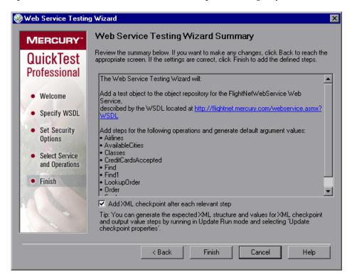
When working with tests, you can automatically insert XML checkpoints by selecting **Add XML checkpoint after each relevant step** (selected by default). Selecting this check box adds an XML checkpoint for each step in the test that has a return value or an output argument. For more information about XML checkpoints, refer to the *QuickTest Professional User's Guide*.
