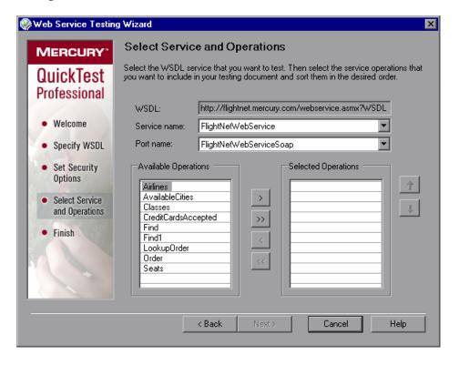
From the **Service name** list and **Port name** list, select the service and port that you want to test. The name of the service you select is also used as the default name of the created test object. If a description of the Web service is available, it is displayed as a tooltip when the cursor is positioned over the service name.
