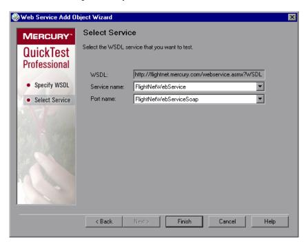
From the **Service name** list and the **Port name** list, select the service and port that you want to test and click **Finish**. The wizard adds a WebService test object to the object repository, representing the specific Web service and port. If a description of the Web service is available, it is displayed as a tooltip when the cursor is positioned over the service name.
