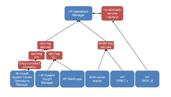
Figure 5: Event integration technology used by some of the existing integration packages for HP Operations Manager
