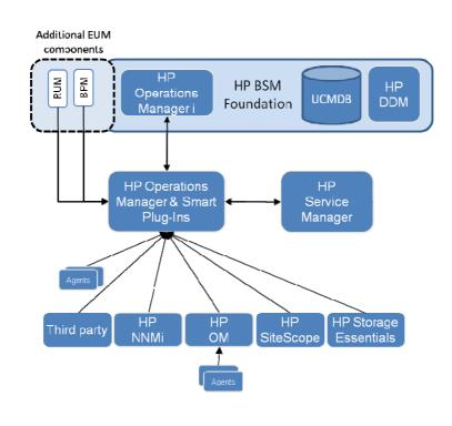
Figure 2: A typical HP BSM solution deployment with HP OMi
