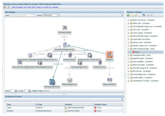
Once saved, this new correlation rule will properly identify a "Node Down" event sent by NNMi for the Exchange Mail Hub server as the root cause event, when at the same time (or within the TBEC correlation time window) the MS Exchange Smart Plug-In for HPOM generates an event indicating that the server's "Mail Flow Status" is "Down".
