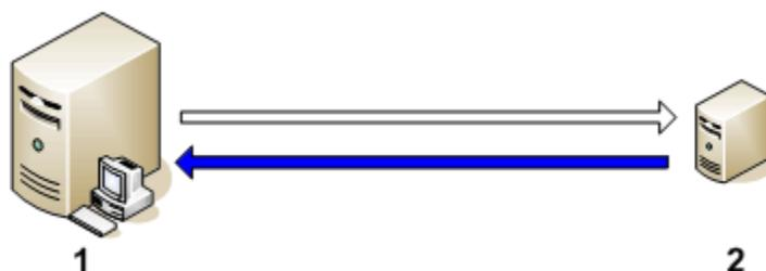
If a firewall blocks inbound HTTPS connections from a node to a management server, the node cannot communicate with the management server properly. To enable proper communication, you configure an HTTPS agent to act as a reverse channel proxy (RCP).
