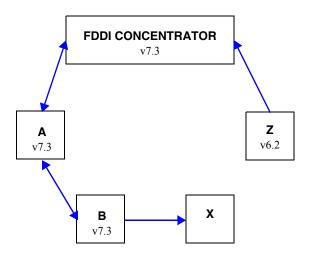
The only way for the ring to remain unbroken is for the next object upstream (Z) to be able to look back downstream and ask object X about itself. If Z supports only SMT v6.2, then Z cannot see downstream, and therefore the ring cannot be closed.
