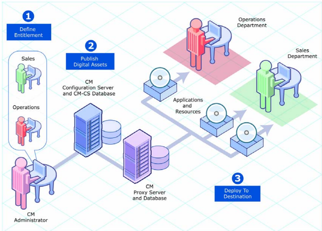
Figure 1 CM infrastructure using CM Proxy Server
