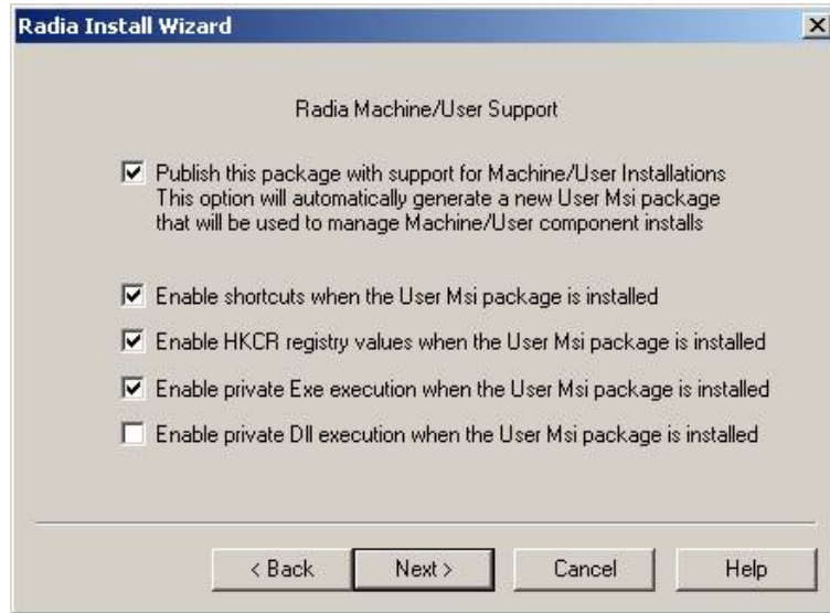
Figure 5.131 ~ With Radia 3.x, use the Radia Install Wizard's option to publish an MSI with support for Machine/User Installations.
