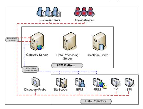
Communication channels between BSM servers, data collectors, application users, and BSM platform components use various protocols on specific ports. For details, see "Port Usage" in the *Platform Administration* guide, found in the HP BSM Documentation Library.
