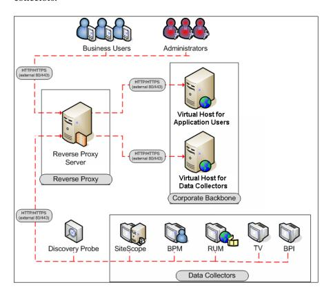
Reverse proxy BSM support should be configured differently in each of the following cases:
