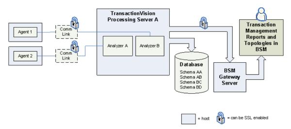
Enabling SSL on the communication link data pathway (left side of the diagram) is dependent on the type of agent and message middleware provider. For more information about enabling SSL on this data pathway, see "Securing with SSL" in the *HP TransactionVision Deployment Guide* PDF.
