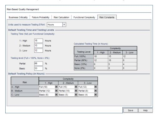
**3** In the **Units used to measure Testing Effort** box, select the unit of measurement that you want Quality Center to display when measuring Testing Time. The available units are **Hours**, **Days**, **Weeks**, and **Months**.
