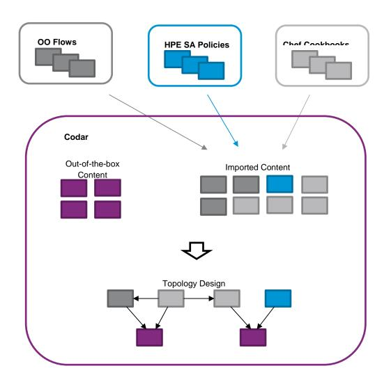
The topology design consists of components connected with relationships. Components represents the final shape of the deployment, and the relationships are dependencies between the components. The designer user just declares *what* should be done and Codar figures out *how* it should be done. The sequence of the tasks is automatically computed based on designed dependencies among components.
