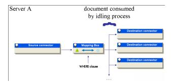
The scenarios running the 3 injectors must not process data at the same time. A filter based on a WHERE clause must be used for each injector to ensure that data is loaded and processed once only.
