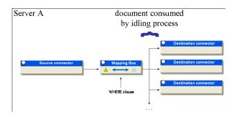
When parallelization is used, several processes run at the same time. A parent process controls its child processes and triggers them when possible.
